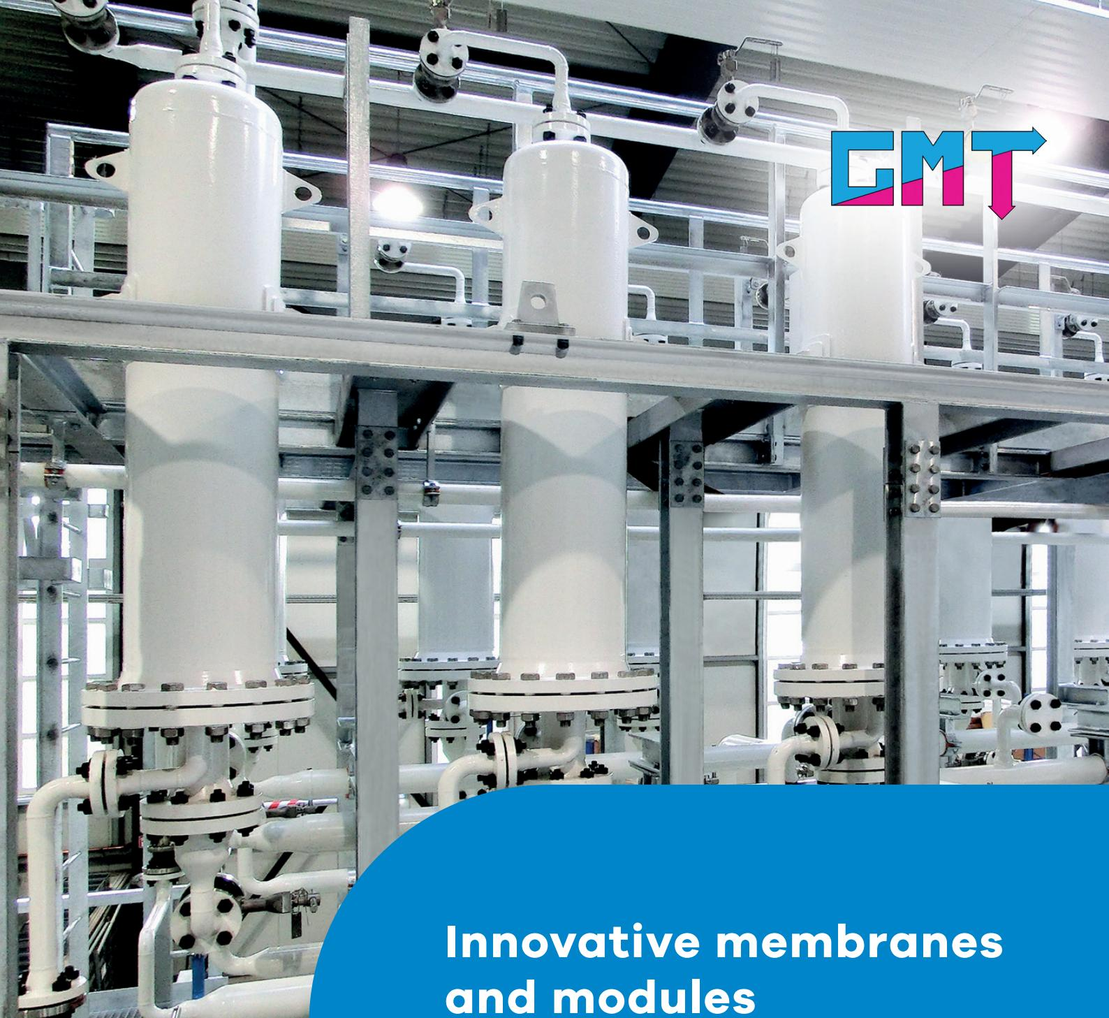
A photograph of a large-scale industrial membrane separation system. The central feature is a row of several large, vertical, white cylindrical modules, likely membrane elements, mounted on a metal frame. They are connected by a complex network of white plastic or metal pipes and valves. The background shows more of the industrial facility, with additional equipment and piping visible through windows in the walls.
